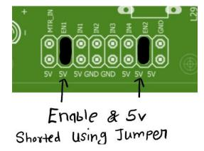
You can use the enable pins to control the speed of the motor by removing the jumper and connecting them to PWM pin.
